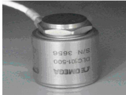
Figure 7. Photo of the force sensor.
