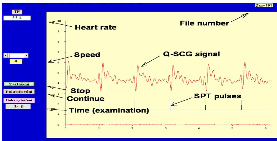
Figure 11. Window during the examination. Q-SCG signal (top), SPT pulses (bottom). Labels with heart rate value, file number, speed and elapsed time are shown and control buttons for Stop and Continue are also inserted. Subject: Male, 59 year.
