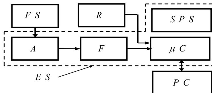
Figure 5. The block diagram of electronic system (ES). A-amplifier, F-bandpass filter, SPS-switching power supply,  $\mu C$ -microcontroller, FS-force sensor, R-receiver (for QRS complex), PC-personal computer.
