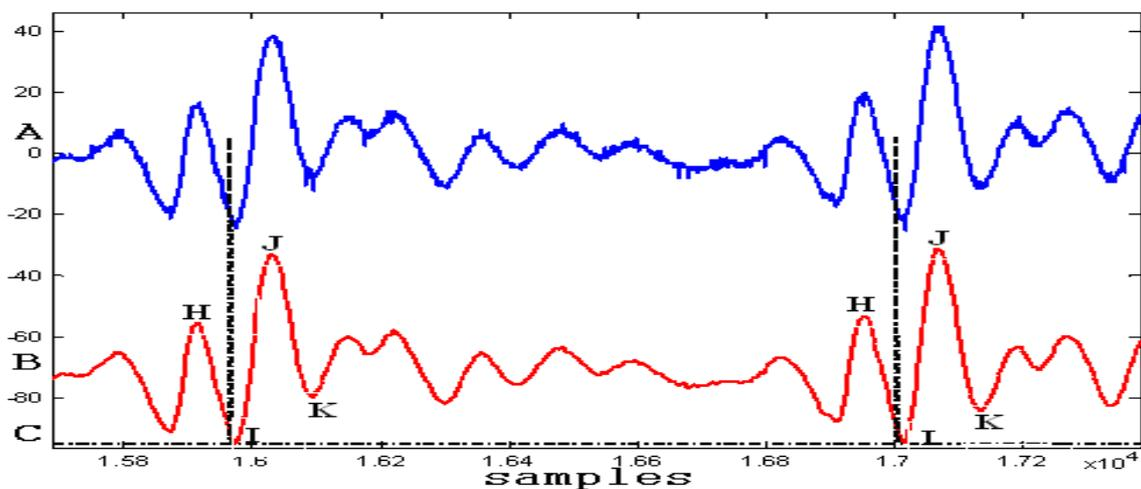
Figure 14. The Q-SCG signal with noise (top), important points of filtered Q-SCG signal (bottom) and SPS pulses (dash). Subject: Male, 59 year.
