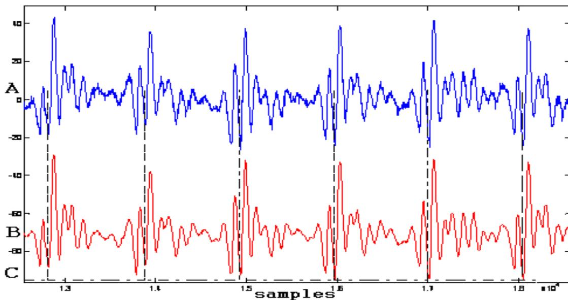
Figure 13. The zoom of Q-SCG raw signal (top), filtered signal (bottom) and SPT pulses (bottom - dash). Subject: Male, 59 year.
