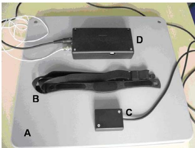
Figure 9. The seismocardiographic system. A-plate with force sensor, B-Sporttester belt (with QRS detector and transmitter), C-receiver, D-electronic system.
