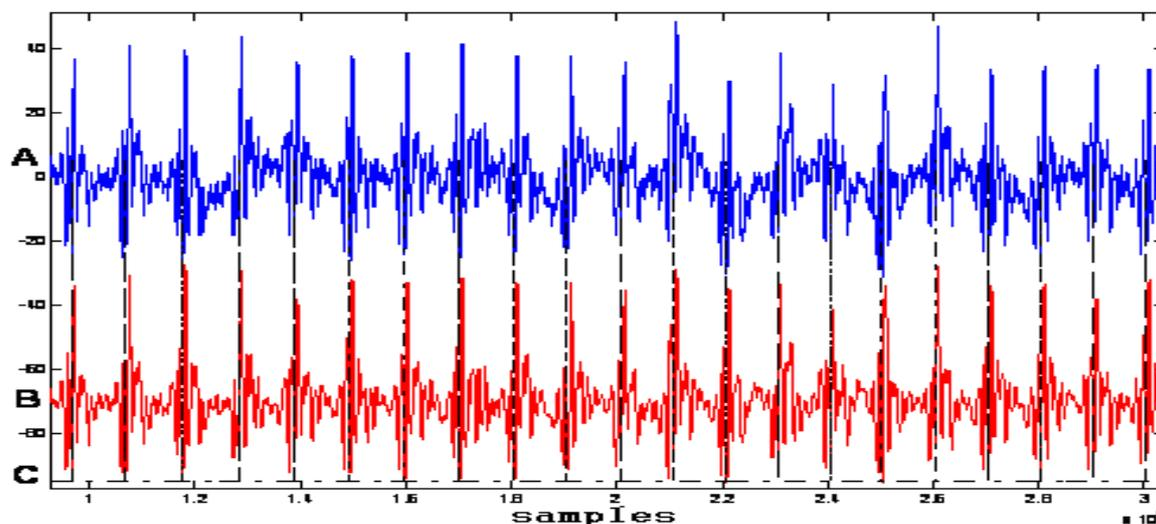
Figure 12. Example of measured and processed signal. The Q-SCG raw signal (top), filtered signal (bottom) and SPT pulses (bottom - dash). Subject: Male, 59 year.
