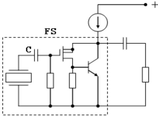
Figure 6. The force sensor DLC101-500 internal circuit.
