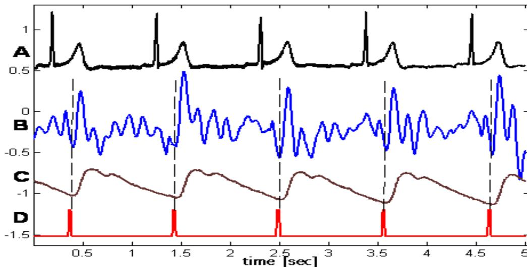
Figure 4. The time diagram of physiological signals. A) ECG signal, B) Q-SCG signal, C) blood pressure waveforms from finger, D) pulses from Sporttester. Subject: Male, 59 year.
