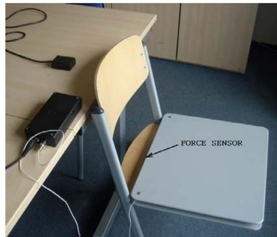
Figure 10. Rigid chair equipped with plate containing force sensor for Q-SCG measuring. Size of the plate is 45x45 cm.
