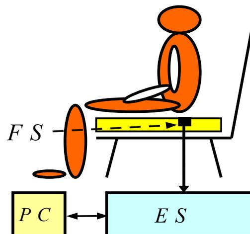
Figure 1. Principle of the convention noninvasive quantitative seismocardiography measuring: FS – Force sensor (piezoelectric transducer), ES - electronic system, PC - personal computer.
