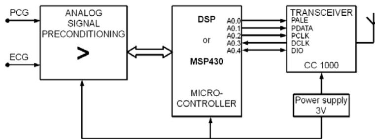
Figure 1. Hardware block diagram
