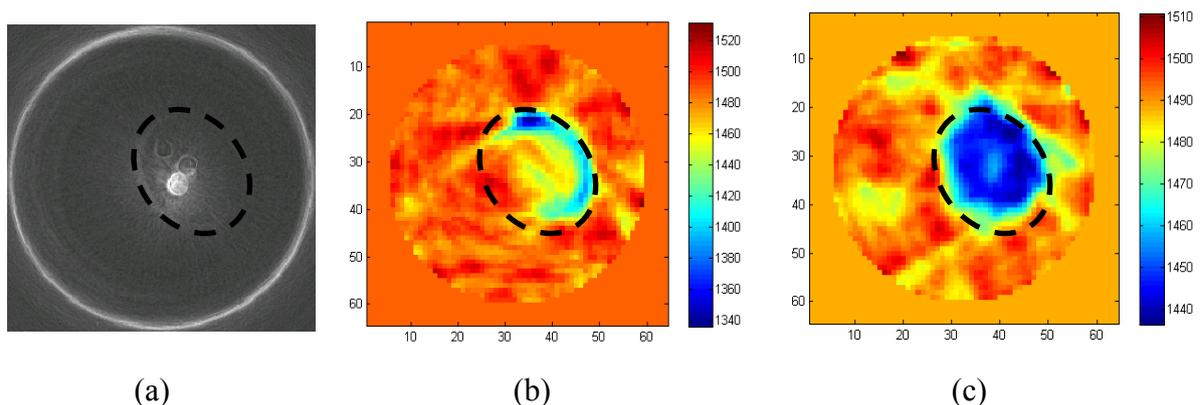
Fig 2. Measured breast phantom image data; black ellipse indicates the breast outline according to the reflectivity image. (a) Reflectivity image. (b) Reconstructed sound-speed image with no focusing. (c) Reconstructed sound-speed image with focusing on the receiver and sender side. Colour-encoded sound-speed values are given in m/s.
