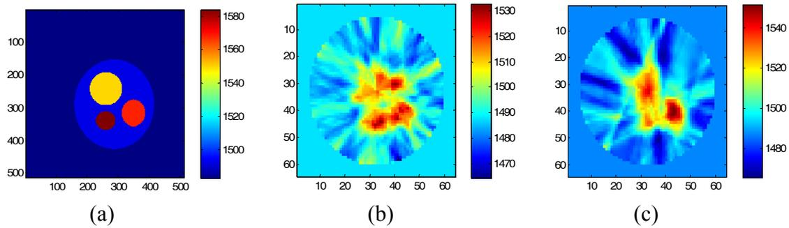
Fig 1. Sound-speed maps for synthetic data (colour-encoded sound-speed values are given in m/s). (a) Reference sound-speed image. (b) Reconstructed sound-speed image with no focusing. (c) Reconstructed sound-speed image with focusing on the receiver and sender side (aperture size: emitter / receiver 32x32/24x24 mm)].
