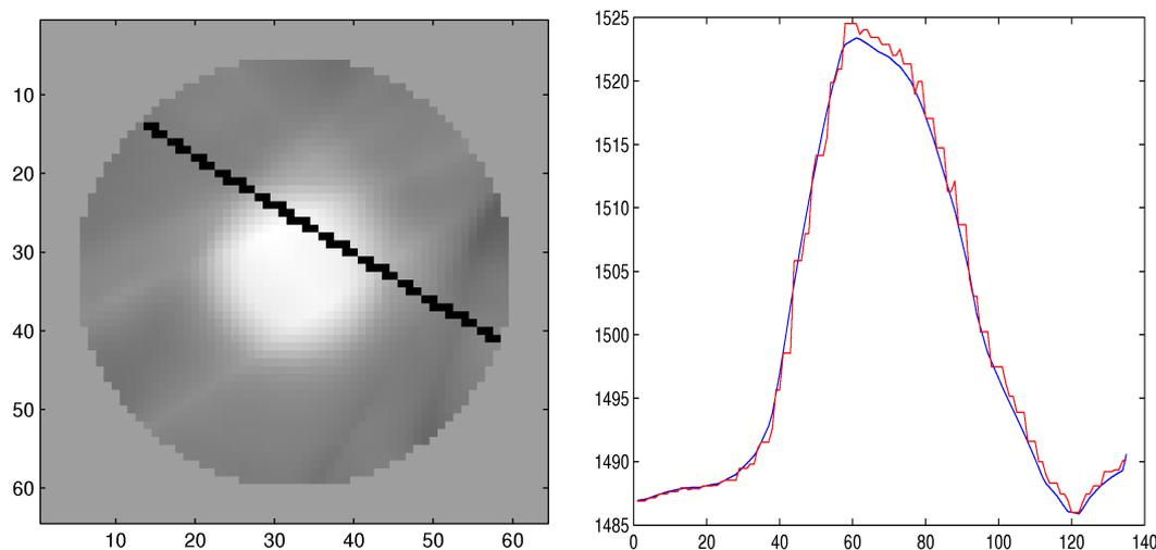
Fig. 4: The results for real phantom simulation of ray propagation. a) the reconstructed SOS map with the pixels hit by simulated ray are marked. b) calculated propagation speed along the simulated ray (blue); again, with input SOS data check (red).
