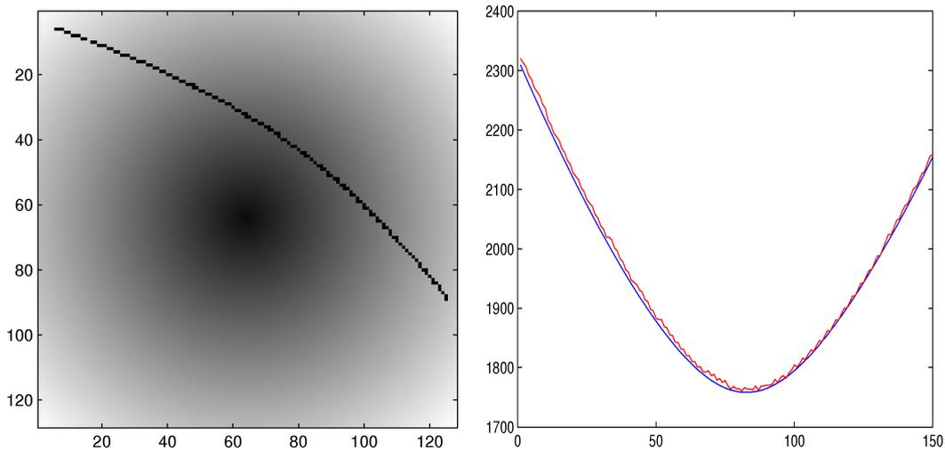
Fig. 3: The results for simulation of ray propagation in artificial configuration. a) the speed of propagation ranging from 1500 m/s to 2405 m/s; the pixels hit by simulated ray are marked. b) a comparison of calculated propagation speed (blue) to input SOS data (red).
