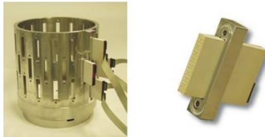
Fig. 1: The USCT experimental setup as developed in KIT, Germany. a) the tank with protrusions to be sealed by individual TASes, b) a TAS.
