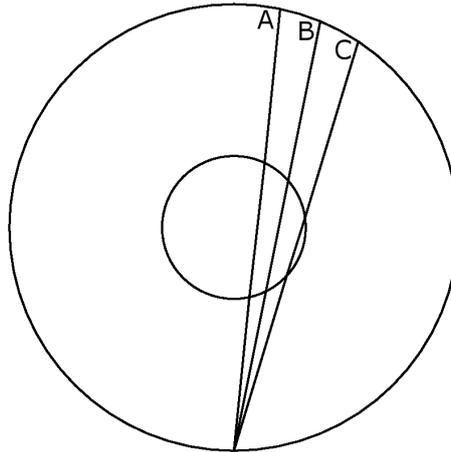
Fig. 2: The geometrical model for the simulated configuration with three selected rays. The outer ring has diameter of 180 mm, the inner one of 64 mm; for further details see below.
